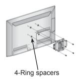
Place the ring spacers on the set before installing the wall mounting bracket so that the inclination of the backside of the set can be adjusted perpendicularly.
